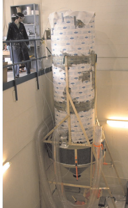
Figure 3.1: Diagram of prototype contactor and photograph of finished structure. Atmospheric \text{CO}_2 is absorbed by NaOH spray. \text{CO}_2 concentration at the air intake and outlet is measured and the rate of \text{CO}_2 absorption is calculated.
